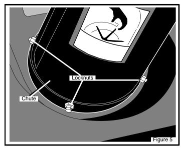
2. Install the **chute** with the bolts and **locknuts**. Make sure the **locknuts** are to the outside as shown.
